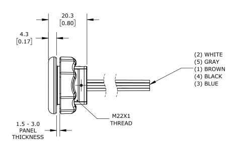
STANDARD CAPACITIVE PUSHBUTTON SENSOR SWITCH, IP69K, 22mm, DYNAMIC, POLYCARBONATE BEZEL, AUTOMATIC LED CONTROL, OPERATOR: BLACK, 30mm, OPERATOR TEXT "POWER SYMBOL", RED/GREEN ILLUMINATED.
