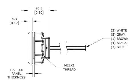
STANDARD CAPACITIVE PUSHBUTTON SENSOR SWITCH, IP69K, 22mm, DYNAMIC, POLYCARBONATE BEZEL, AUTOMATIC LED CONTROL, OPERATOR: BLACK, 30mm, OPERATOR TEXT "RESET", BLUE ILLUMINATED.
