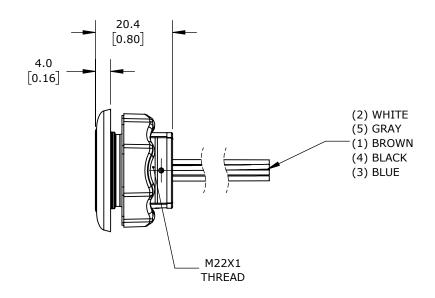
CAPTRON CANEO SERIES10 HYGIENIC CAPACITIVE PUSHBUTTON SENSOR SWITCH, IP69K, 22mm, STATIC, STAINLESS STEEL BEZEL, SEMI-AUTOMATIC LED CONTROL, OPERATOR: WHITE, 32.4mm.
