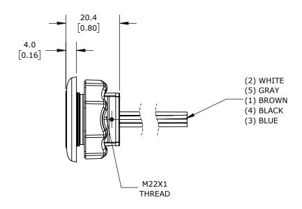
CAPTRON CANEO SERIES10 HYGIENIC CAPACITIVE PUSHBUTTON SENSOR SWITCH, IP69K, 22mm, STATIC, STAINLESS STEEL BEZEL, AUTOMATIC LED CONTROL, OPERATOR: WHITE, 32.4mm, OPERATOR TEXT "RESET", WHITE.
