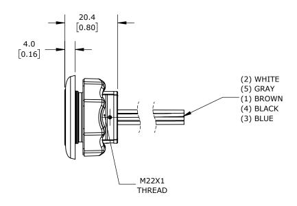
HYGIENIC CAPACITIVE PUSHBUTTON SENSOR SWITCH, IP69K, 22mm, STATIC, STAINLESS STEEL BEZEL, SEMI-AUTOMATIC LED CONTROL, OPERATOR: WHITE, 32.4mm, OPERATOR TEXT "POWER SYMBOL", WHITE.
