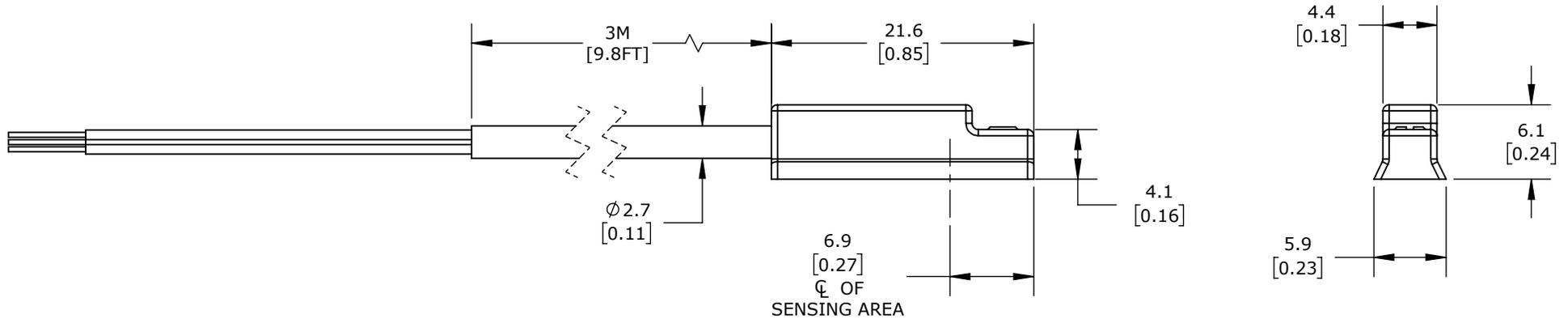
DOVETAIL, PNP, N.O. OUTPUT, 5-28 VDC OPERATING VOLTAGE, LED INDICATION, 9.8FT (3.00m) 3-WIRE PIGTAIL WITH WIRE LEADS, STRAIGHT CABLE ENTRY, 1/4IN 60 DEGREE DOVETAIL SLOT MOUNT, FOR POSITION SENSING.
