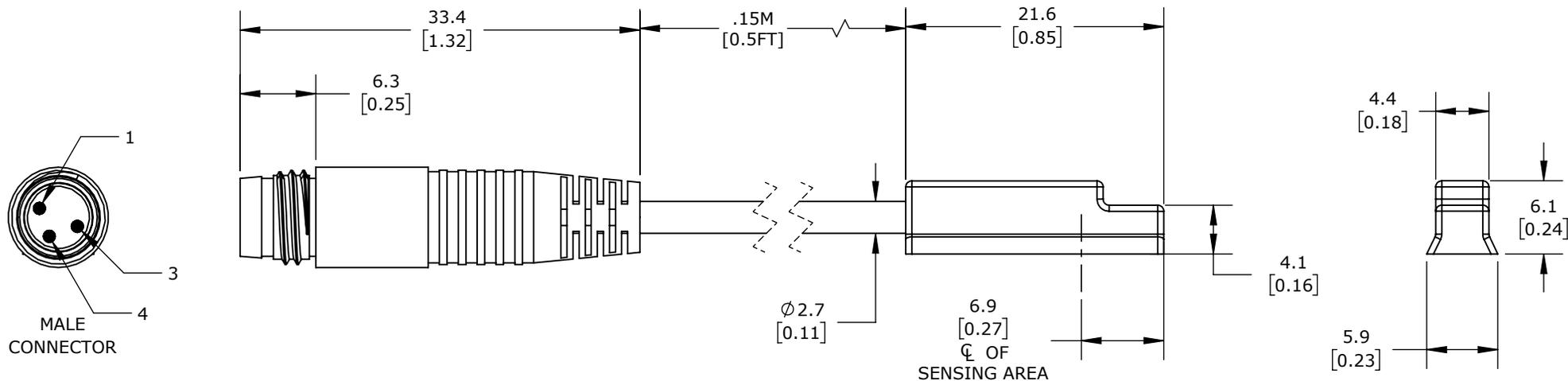
DOVETAIL, NPN, N.O. OUTPUT, 5-28 VDC OPERATING VOLTAGE, LED INDICATION, 0.5FT (0.15m) CABLE WITH 3-PIN M8 SNAP-FIT CONNECTOR, STRAIGHT CABLE ENTRY, 1/4IN 60 DEGREE DOVETAIL SLOT MOUNT, FOR POSITION SENSING.
