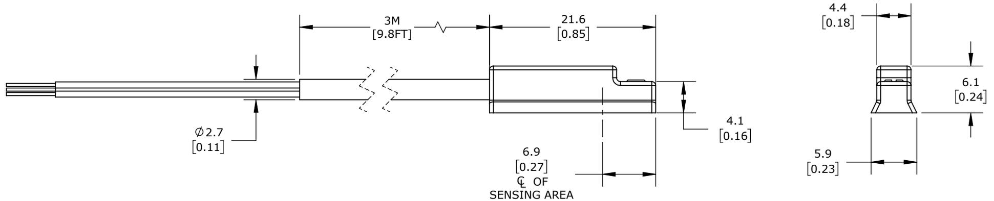
DOVETAIL, NPN, N.O. OUTPUT, 5-28 VDC OPERATING VOLTAGE, LED INDICATION, 9.8FT (3.00m) 3-WIRE PIGTAIL WITH WIRE LEADS, STRAIGHT CABLE ENTRY, 1/4IN 60 DEGREE DOVETAIL SLOT MOUNT, FOR POSITION SENSING.
