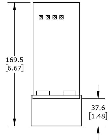
WEG ELECTRIC EMI INPUT FILTER, 3-PHASE, 8.2A, 35mm DIN RAIL MOUNT, EMI/RFI FILTERING,
