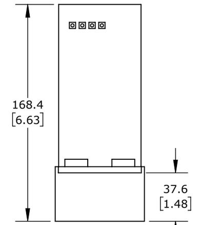
WEG ELECTRIC EMI INPUT FILTER, 3-PHASE, 15.2A, 35mm DIN RAIL MOUNT, EMI/RFI FILTERING,
