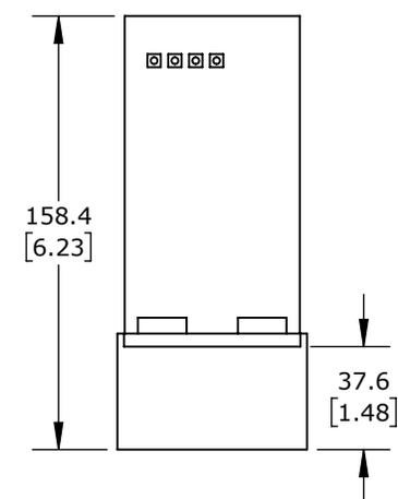
WEG ELECTRIC EMI INPUT FILTER, 3-PHASE, 7.3A, 35mm DIN RAIL MOUNT, EMI/RFI FILTERING,
