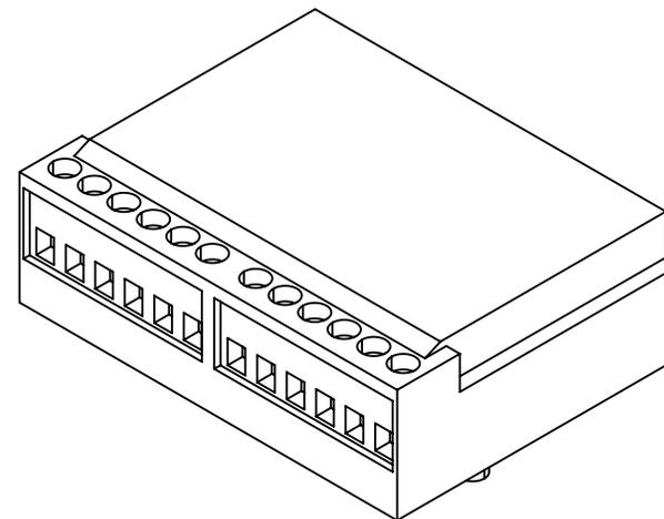
WEG ELECTRIC CFW320 SERIES ENCODER ANALOG COMBO MODULE, 400 KHZ MAXIMUM SWITCHING FREQUENCY, 1-CHANNEL QUADRATURE ENCODER INPUT, ANALOG INPUT: 1-CHANNEL, ANALOG OUTPUT: 2-CHANNEL, FOR USE WITH WEG CFW320 SERIES AC DRIVES
