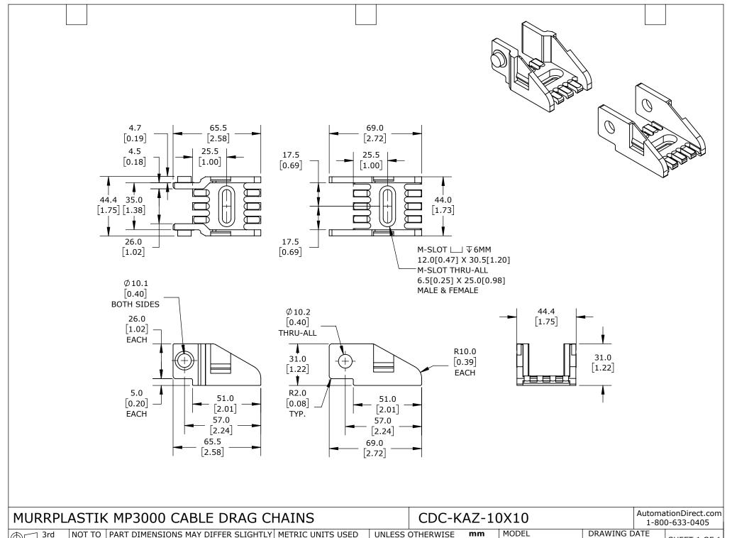
PART DIMENSIONS MAY DIFFER SLIGHTLY METRIC UNITS USED ANGLE SCALE
