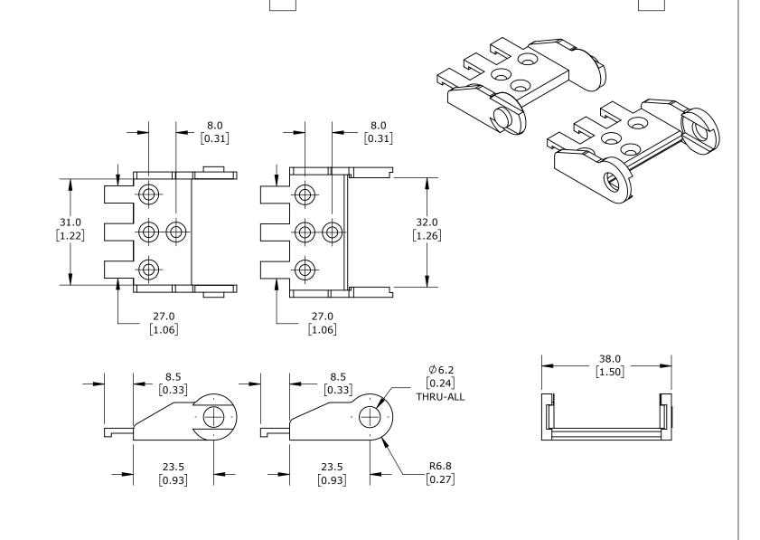
0.39IN INSIDE HEIGHT, 1.22IN INSIDE WIDTH, POLYAMIDE, BLACK. FOR USE WITH MP10 SERIES ENERGY CHAIN.
