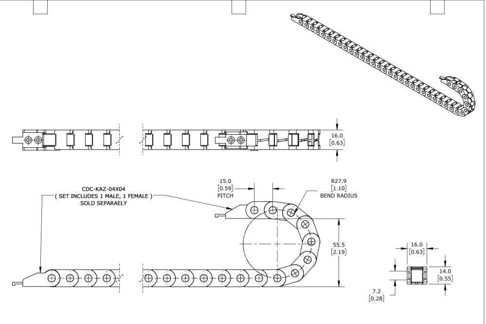
0.39IN INSIDE HEIGHT, 0.35IN INSIDE WIDTH, 1.1IN BEND RADIUS, OUTSIDE OPENING, 0.59IN PITCH, 1.6FT/0.5M LENGTH, BLACK. REQUIRES CDC-KAZ-04X04 BRACKET FOR MOUNTING.
