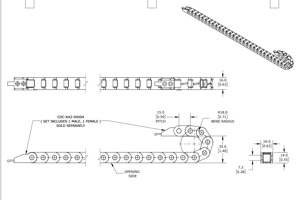
0.39IN INSIDE HEIGHT, 0.35IN INSIDE WIDTH, 0.71IN BEND RADIUS, OUTSIDE OPENING, 0.59IN PITCH, 1.6FT/0.5M LENGTH, BLACK. REQUIRES CDC-KAZ-04X04 BRACKET FOR MOUNTING.
