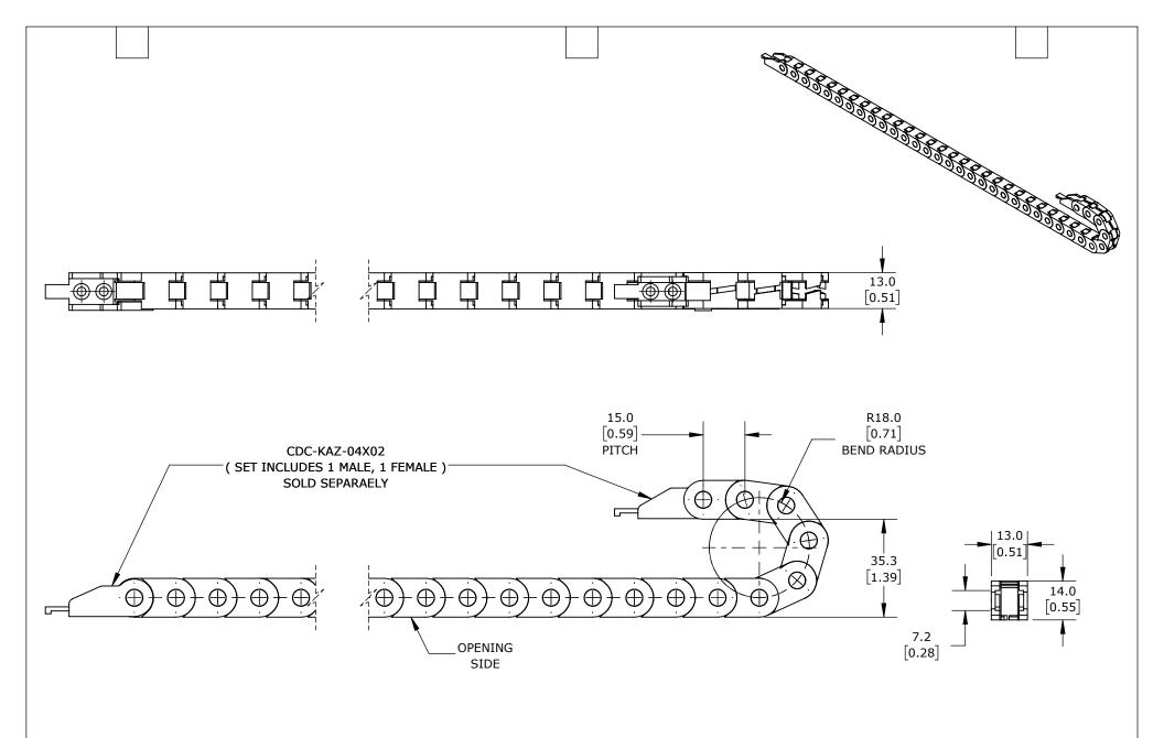
0.39IN INSIDE HEIGHT, 0.24IN INSIDE WIDTH, 0.71IN BEND RADIUS, OUTSIDE OPENING, 0.59IN PITCH, 1.6FT/0.5M LENGTH, BLACK. REQUIRES CDC-KAZ-04X02 BRACKET FOR MOUNTING.
