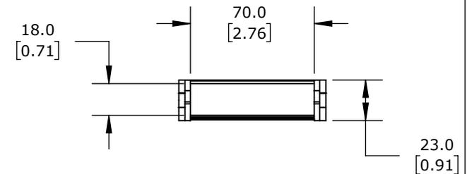
0.71IN INSIDE HEIGHT, 2.76IN INSIDE WIDTH, 3.07IN BEND RADIUS, INSIDE OPENING, 1.3IN PITCH, 3.2FT/1m LENGTH, BLACK. REQUIRES CDC-KAZ-0.7X2.8 BRACKET FOR MOUNTING.
