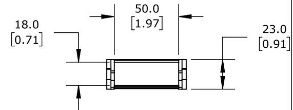
0.71IN INSIDE HEIGHT, 1.97IN INSIDE WIDTH, 3.07IN BEND RADIUS, OUTSIDE OPENING, 1.3IN PITCH, 3.2FT/1m LENGTH, BLACK. REQUIRES CDC-KAZ-0.7X2.0 BRACKET FOR MOUNTING.
