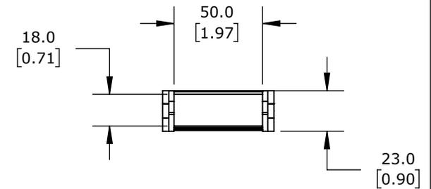
0.71IN INSIDE HEIGHT, 1.97IN INSIDE WIDTH, 1.1IN BEND RADIUS, INSIDE OPENING, 1.3IN PITCH, 3.2FT/1m LENGTH, BLACK. REQUIRES CDC-KAZ-0.7X2.0 BRACKET FOR MOUNTING.
