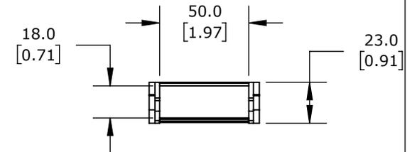
0.71IN INSIDE HEIGHT, 1.97IN INSIDE WIDTH, 1.89IN BEND RADIUS, OUTSIDE OPENING, 1.3IN PITCH, 3.2FT/1m LENGTH, BLACK. REQUIRES CDC-KAZ-0.7X2.0 BRACKET FOR MOUNTING.
