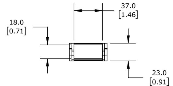
0.71IN INSIDE HEIGHT, 1.46IN INSIDE WIDTH, 3.07IN BEND RADIUS, OUTSIDE OPENING, 1.3IN PITCH, 3.2FT/1m LENGTH, BLACK. REQUIRES CDC-KAZ-0.7X1.5 BRACKET FOR MOUNTING.
