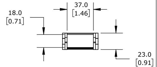
0.71IN INSIDE HEIGHT, 1.46IN INSIDE WIDTH, 3.07IN BEND RADIUS, INSIDE OPENING, 1.3IN PITCH, 3.2FT/1m LENGTH, BLACK. REQUIRES CDC-KAZ-0.7X1.5 BRACKET FOR MOUNTING.
