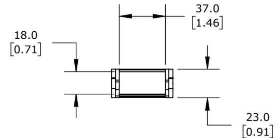
0.71IN INSIDE HEIGHT, 1.46IN INSIDE WIDTH, 1.89IN BEND RADIUS, OUTSIDE OPENING, 1.3IN PITCH, 3.2FT/1m LENGTH, BLACK. REQUIRES CDC-KAZ-0.7X1.5 BRACKET FOR MOUNTING.
