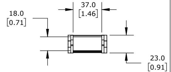
0.71IN INSIDE HEIGHT, 1.46IN INSIDE WIDTH, 1.89IN BEND RADIUS, INSIDE OPENING, 1.3IN PITCH, 3.2FT/1m LENGTH, BLACK. REQUIRES CDC-KAZ-0.7X1.5 BRACKET FOR MOUNTING.
