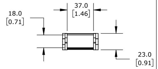
0.71IN INSIDE HEIGHT, 1.46IN INSIDE WIDTH, 1.5IN BEND RADIUS, INSIDE OPENING, 1.3IN PITCH, 3.2FT/1m LENGTH, BLACK. REQUIRES CDC-KAZ-0.7X1.5 BRACKET FOR MOUNTING.
