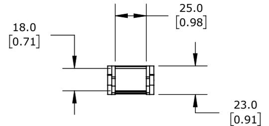
0.71IN INSIDE HEIGHT, 0.98IN INSIDE WIDTH, 3.07IN BEND RADIUS, OUTSIDE OPENING, 1.3IN PITCH, 3.2FT/1m LENGTH, BLACK. REQUIRES CDC-KAZ-0.7X1.0 BRACKET FOR MOUNTING.
