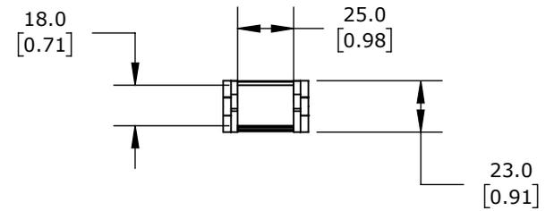
0.71IN INSIDE HEIGHT, 0.98IN INSIDE WIDTH, 3.07IN BEND RADIUS, INSIDE OPENING, 1.3IN PITCH, 3.2FT/1m LENGTH, BLACK. REQUIRES CDC-KAZ-0.7X1.0 BRACKET FOR MOUNTING.
