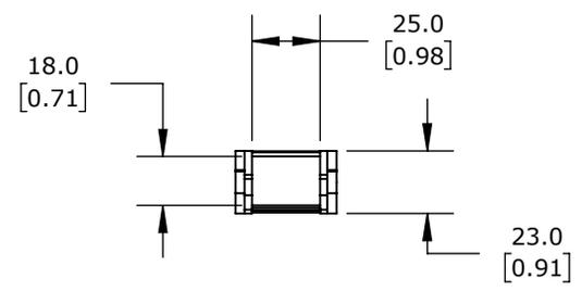
0.71IN INSIDE HEIGHT, 0.98IN INSIDE WIDTH, 1.89IN BEND RADIUS, OUTSIDE OPENING, 1.3IN PITCH, 3.2FT/1m LENGTH, BLACK. REQUIRES CDC-KAZ-0.7X1.0 BRACKET FOR MOUNTING.
