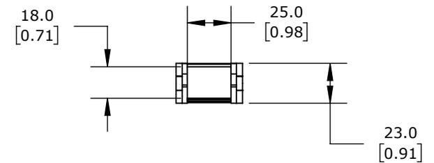
0.71IN INSIDE HEIGHT, 0.98IN INSIDE WIDTH, 1.89IN BEND RADIUS, INSIDE OPENING, 1.3IN PITCH, 3.2FT/1m LENGTH, BLACK. REQUIRES CDC-KAZ-0.7X1.0 BRACKET FOR MOUNTING.
