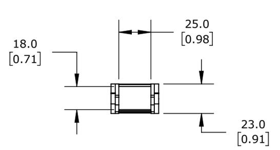
0.71IN INSIDE HEIGHT, 0.98IN INSIDE WIDTH, 1.5IN BEND RADIUS, OUTSIDE OPENING, 1.3IN PITCH, 3.2FT/1m LENGTH, BLACK. REQUIRES CDC-KAZ-0.7X1.0 BRACKET FOR MOUNTING.
