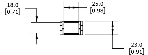
0.71IN INSIDE HEIGHT, 0.98IN INSIDE WIDTH, 1.5IN BEND RADIUS, INSIDE OPENING, 1.3IN PITCH, 3.2FT/1m LENGTH, BLACK. REQUIRES CDC-KAZ-0.7X1.0 BRACKET FOR MOUNTING.
