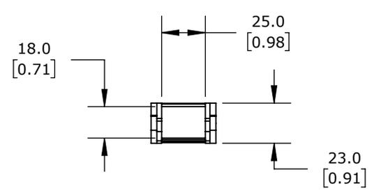
0.71IN INSIDE HEIGHT, 0.98IN INSIDE WIDTH, 1.1IN BEND RADIUS, OUTSIDE OPENING, 1.3IN PITCH, 3.2FT/1m LENGTH, BLACK. REQUIRES CDC-KAZ-0.7X1.0 BRACKET FOR MOUNTING.
