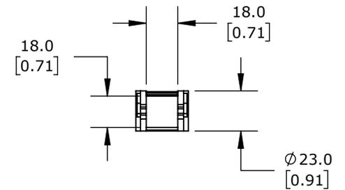
0.71IN INSIDE HEIGHT, 0.71IN INSIDE WIDTH, 3.07IN BEND RADIUS, OUTSIDE OPENING, 1.3IN PITCH, 3.2FT/1m LENGTH, BLACK. REQUIRES CDC-KAZ-0.7X0.7 BRACKET FOR MOUNTING.
