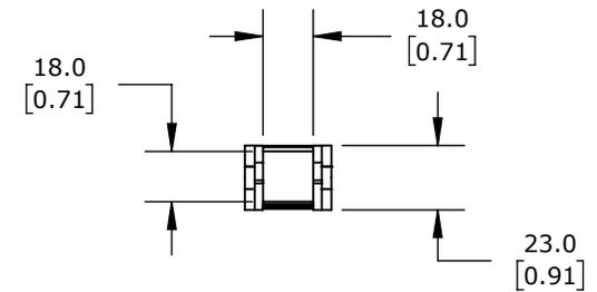
0.71IN INSIDE HEIGHT, 0.71IN INSIDE WIDTH, 3.07IN BEND RADIUS, INSIDE OPENING, 1.3IN PITCH, 3.2FT/1m LENGTH, BLACK. REQUIRES CDC-KAZ-0.7X0.7 BRACKET FOR MOUNTING.
