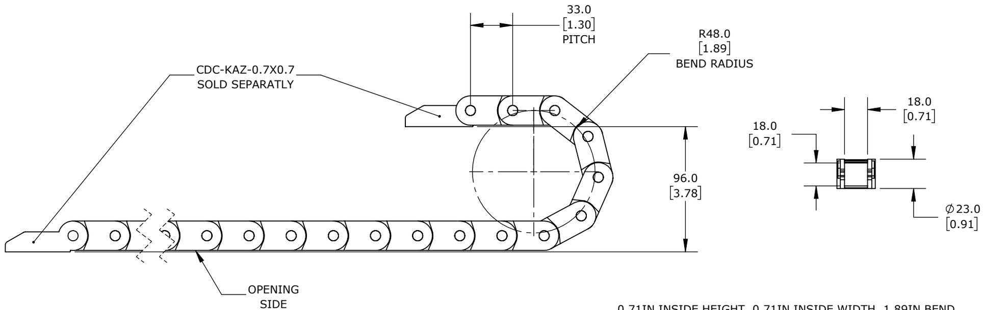
0.71IN INSIDE HEIGHT, 0.71IN INSIDE WIDTH, 1.89IN BEND RADIUS, OUTSIDE OPENING, 1.3IN PITCH, 3.2FT/1m LENGTH, BLACK. REQUIRES CDC-KAZ-0.7X0.7 BRACKET FOR MOUNTING.
