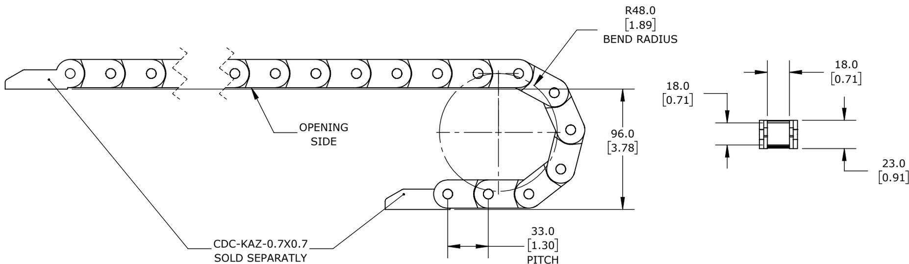
0.71IN INSIDE HEIGHT, 0.71IN INSIDE WIDTH, 1.89IN BEND RADIUS, INSIDE OPENING, 1.3IN PITCH, 3.2FT/1m LENGTH, BLACK. REQUIRES CDC-KAZ-0.7X0.7 BRACKET FOR MOUNTING.
