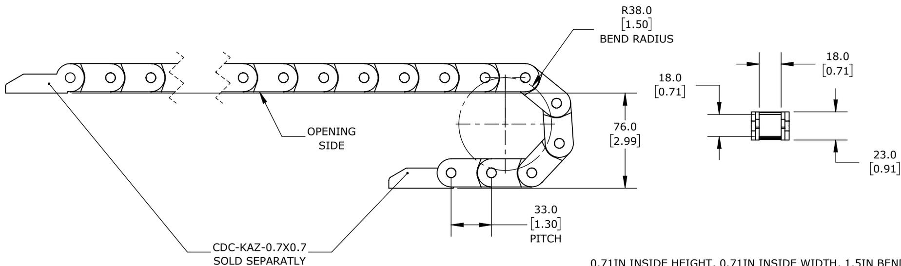
0.71IN INSIDE HEIGHT, 0.71IN INSIDE WIDTH, 1.5IN BEND RADIUS, INSIDE OPENING, 1.3IN PITCH, 3.2FT/1m LENGTH, BLACK. REQUIRES CDC-KAZ-0.7X0.7 BRACKET FOR MOUNTING.
