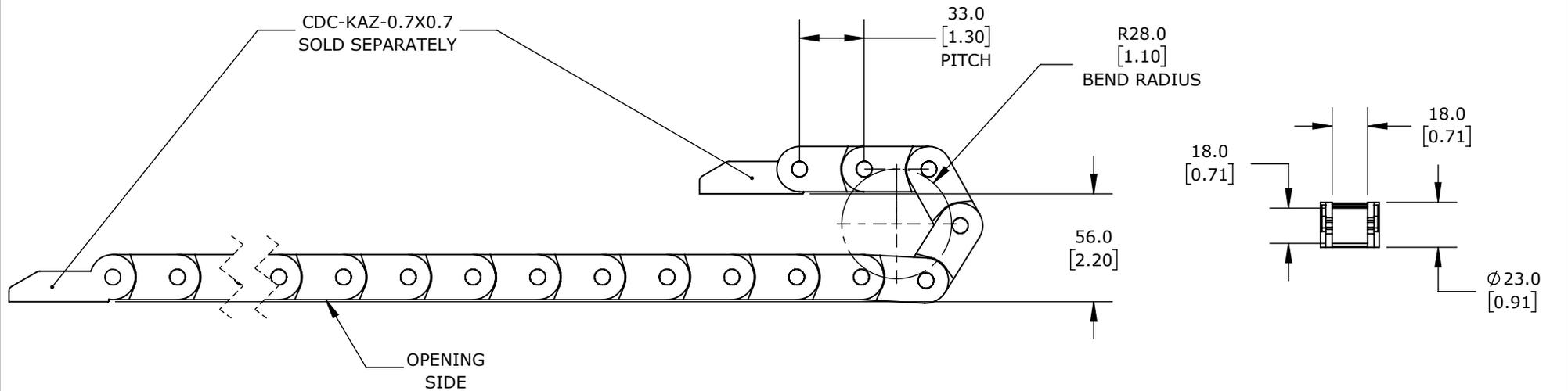
0.71IN INSIDE HEIGHT, 0.71IN INSIDE WIDTH, 1.1IN BEND RADIUS, OUTSIDE OPENING, 1.3IN PITCH, 3.2FT/1m LENGTH, BLACK. REQUIRES CDC-KAZ-0.7X0.7 BRACKET FOR MOUNTING.
