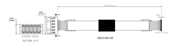
CABLE / LEAD WIRE SHIELDED CABLE WITH 10 WIRES AWG 24 AND UL MARKED
