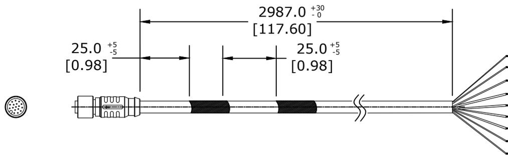
DATALOGIC CABLE, CONNECTION, M12 AXIAL FEMALE TO PIGTAIL, 17-POLE, PVC, 9.8FT/3M CABLE LENGTH.
