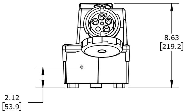
LOAD BREAK CAPABLE, 3-POLE, 600 VAC, 60A, 3-PHASE, 3-POLE, 4-WIRE, 9 HOUR PIN AND SLEEVE RECEPTACLE, 10KA SCCR, 11.9IN X6.9IN X8.6IN HOUSING.
