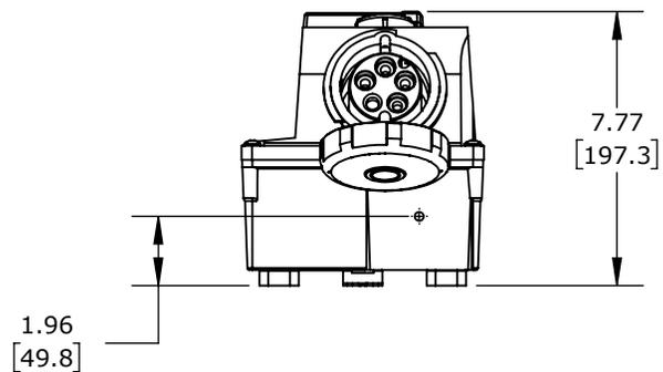
LOAD BREAK CAPABLE, 3-POLE, 600 VAC, 30A, 3-PHASE, 4-POLE, 5-WIRE, 7 HOUR PIN AND SLEEVE RECEPTACLE, 10KA SCCR, 10.1IN X6.9IN X7.8IN HOUSING.
