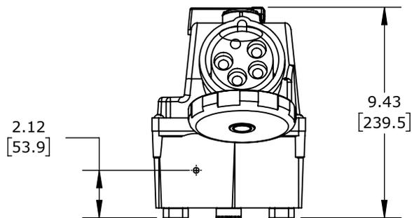
LOAD BREAK CAPABLE, 3-POLE, 600 VAC, 100A, 3-PHASE, 4-POLE, 5-WIRE, 9 HOUR PIN AND SLEEVE RECEPTACLE, 10KA SCCR, 11.9IN X6.9IN X9.3IN HOUSING.
