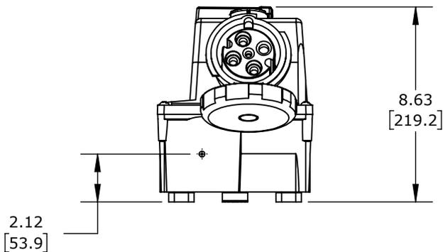
LOAD BREAK CAPABLE, 3-POLE, 600 VAC, 60A, 3-PHASE, 3-POLE, 4-WIRE, 9 HOUR PIN AND SLEEVE RECEPTACLE, 10KA SCCR, 11.9IN X6.9IN X8.6IN HOUSING.
