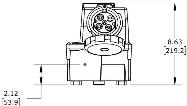
LOAD BREAK CAPABLE, 3-POLE, 600 VAC, 60A, 3-PHASE, 3-POLE, 4-WIRE, 5 HOUR PIN AND SLEEVE RECEPTACLE, 10KA SCCR, 11.9IN X6.9IN X8.6IN HOUSING.
