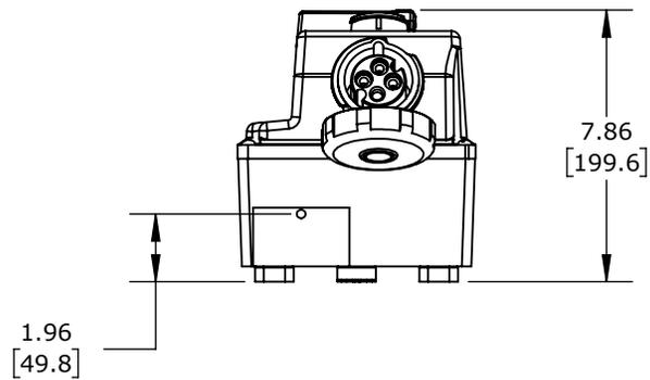
LOAD BREAK CAPABLE, 3-POLE, 600 VAC, 30A, 1-PHASE, 3-POLE, 4-WIRE, 12 HOUR PIN AND SLEEVE RECEPTACLE, 10KA SCCR, 10.1IN X6.9IN X7.8IN HOUSING.
