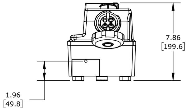
ROTARY ENCLOSED, LOAD BREAK CAPABLE, 3-POLE, 600 VAC, 20A, 3-PHASE, 3-POLE, 4-WIRE, 9 HOUR PIN AND SLEEVE RECEPTACLE, 10KA SCCR, 10.1IN X6.9IN X7.8IN HOUSING.
