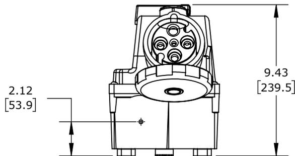
LOAD BREAK CAPABLE, 3-POLE, 600 VAC, 100A, 3-PHASE, 3-POLE, 4-WIRE, 9 HOUR PIN AND SLEEVE RECEPTACLE, 10KA SCCR, 11.9IN X6.9IN X9.3IN HOUSING.
