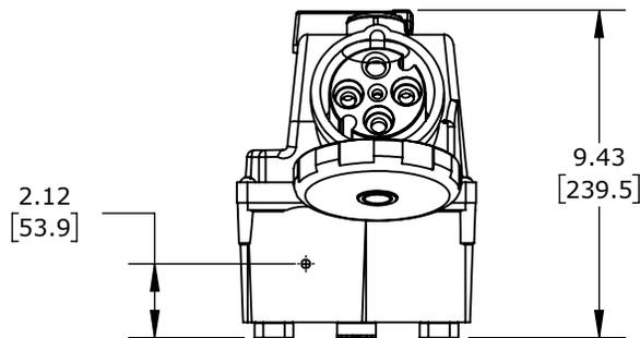
LOAD BREAK CAPABLE, 3-POLE, 600 VAC, 100A, 3-PHASE, 3-POLE, 4-WIRE, 7 HOUR PIN AND SLEEVE RECEPTACLE, 10KA SCCR, 11.9IN X6.9IN X9.3IN HOUSING.
